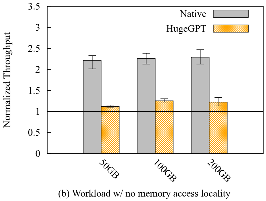
Figure 2.1: Throughputs of native system, and HugeGPT. Throughputs are normalized to vanilla Linux/KVM.
