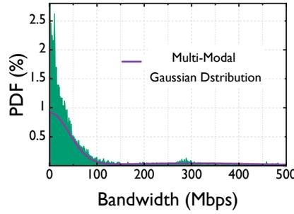
Figure 18: Probability distribution for 4G access bandwidths.
