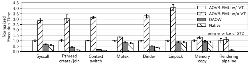
Figure 18: Micro-benchmark results of various key operations in AOVB-EMU, DAOW, and native Android-x86.
